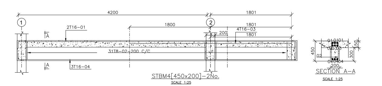
1. All dimensions are in millimetres unless otherwise stated. 2. All reinforcements must be checked and approved by project structural engineer
