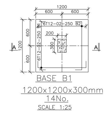
Bearing capacity=200KN/M2 MURRAM SOIL
