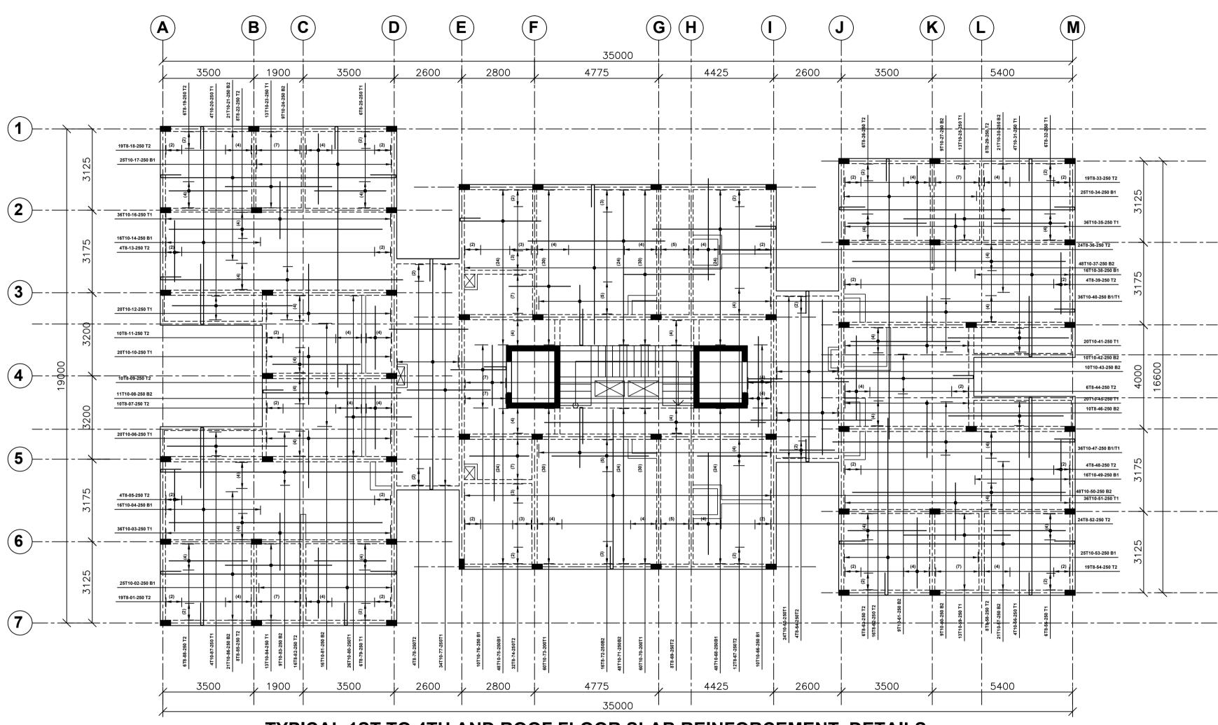
TYPICAL 1ST TO 4TH AND ROOF FLOOR SLAB REINFORCEMENT DETAILS The Slab is 150mm Thick Suspended RC Slab
