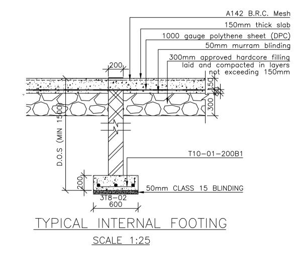
Bearing capacity=350KN/M2 ROCK
