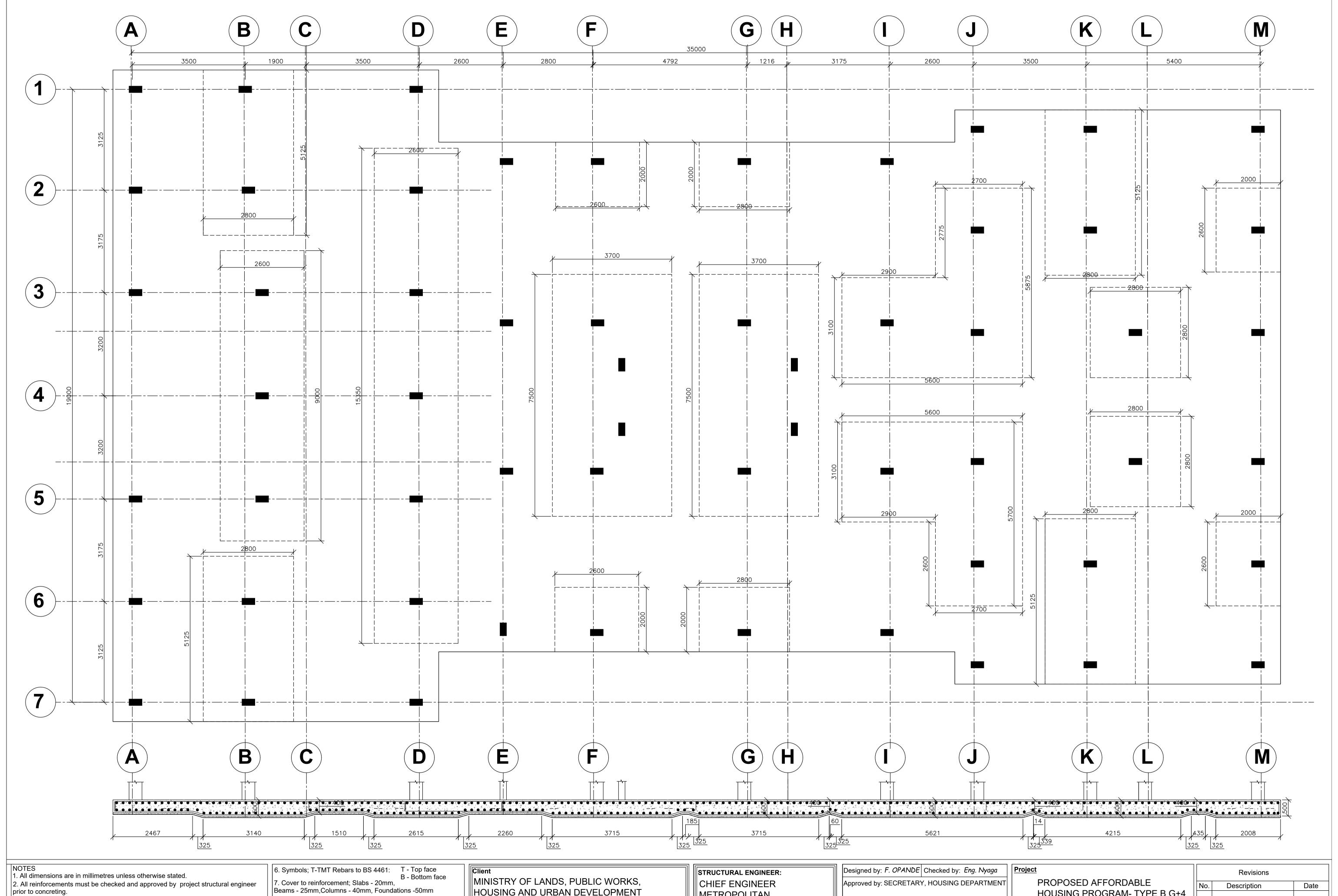
3. All reinforced concrete to be Class 25 mix and blinding concrete to be Class 15 mix. 4. Only figured dimensions to be taken from this drawing.
