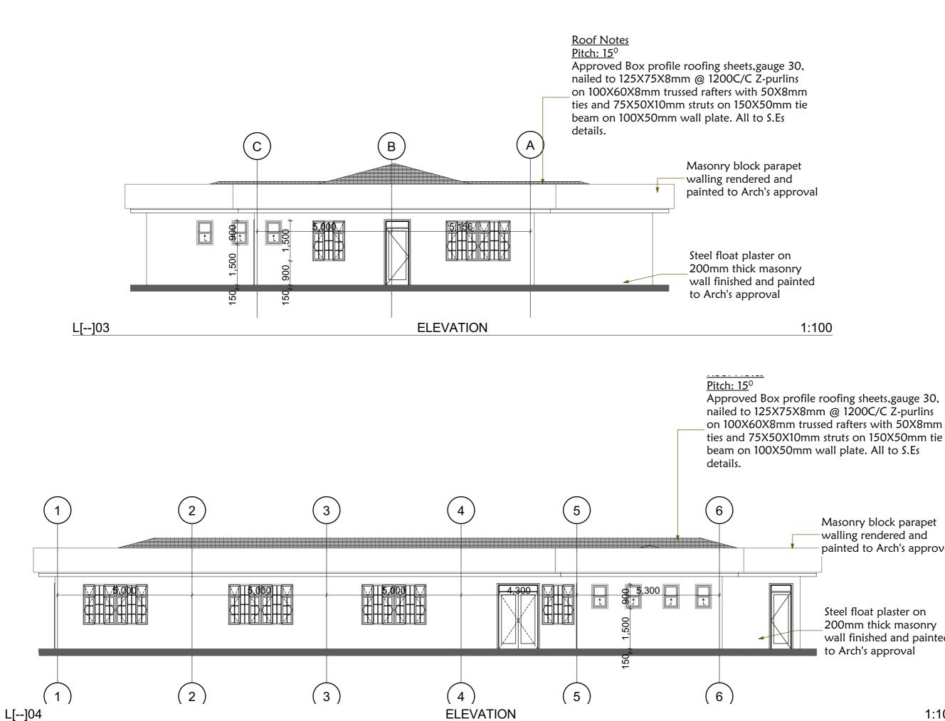
Masonry block parapet walling rendered and painted to Arch's approval
