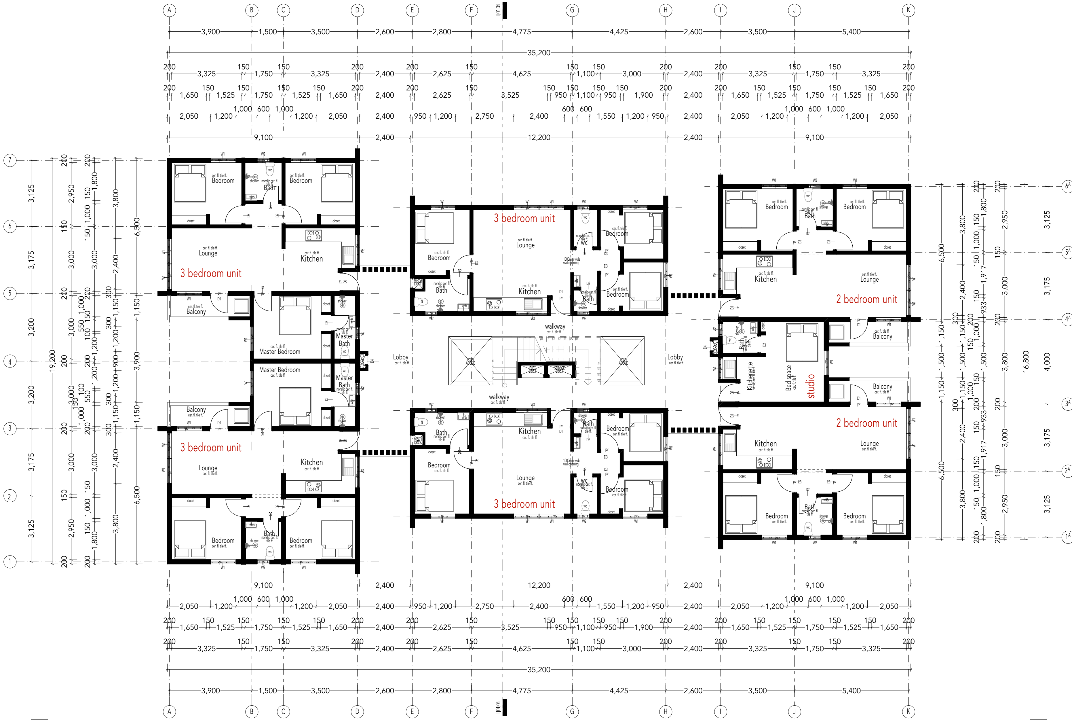
LQ10102 TYPICAL UPPER FLOOR PLAN scale 1:100 PLINTH 530 sqm.
