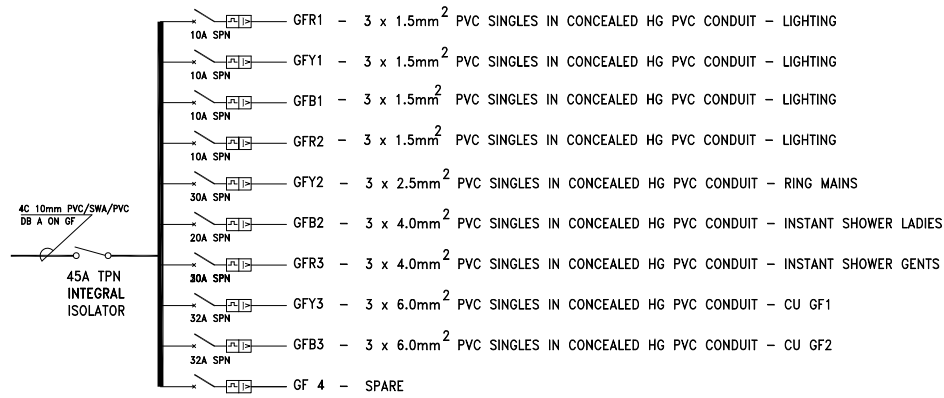
4 WAY DISTRIBUTION BOARD 'GF' SURFACE MOUNTED IN ATTENDANT'S OFFICE WITH INTEGRAL 45A TPN ISOLATOR AND COVER AS SCHNEIDER FOR CIRCUITS GROUND FLOOR
