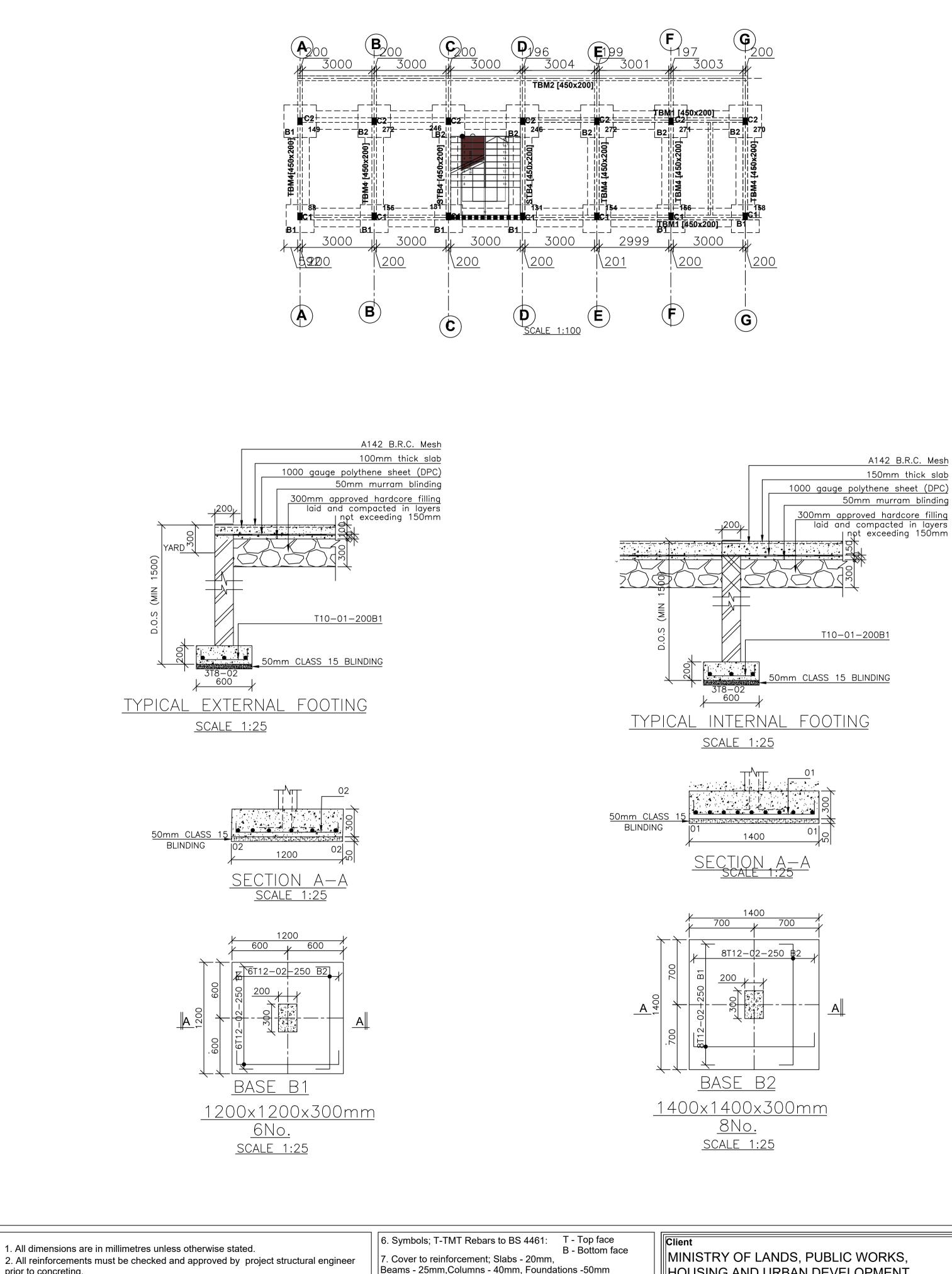
prior to concreting. 3. All reinforced concrete to be Class 25 mix and blinding concrete to be Class 15 mix. 8. All structural steel be grade 43A. 4. Only figured dimensions to be taken from this drawing. 5. Any descripancy indimensions to be reported to the project consultants i.e architect or engineer.
