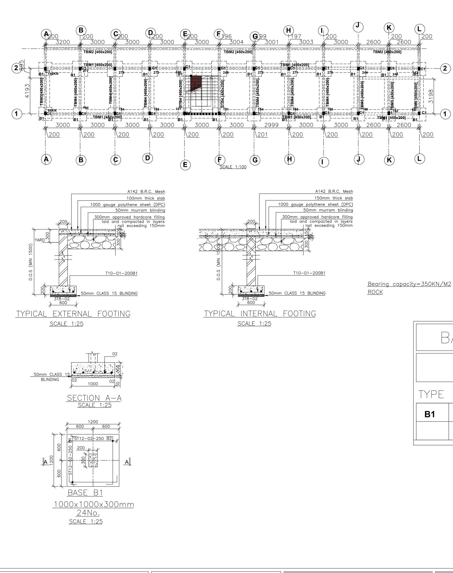
1. All dimensions are in millimetres unless otherwise stated. 2. All reinforcements must be checked and approved by project structural engineer prior to concreting.
