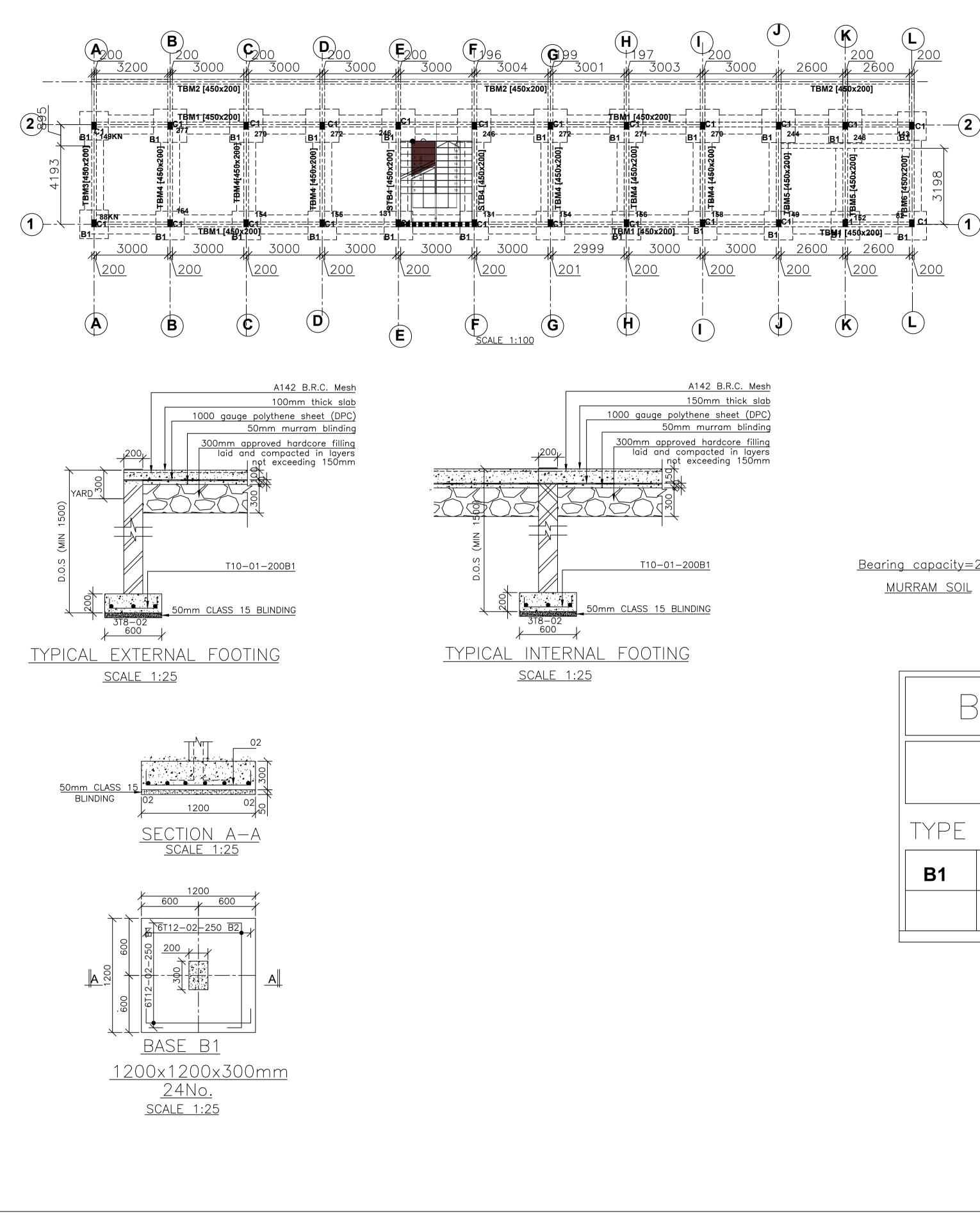
1. All dimensions are in millimetres unless otherwise stated. 2. All reinforcements must be checked and approved by project structural engineer prior to concreting. 3. All reinforced concrete to be Class 25 mix and blinding concrete to be Class 15 mix.
