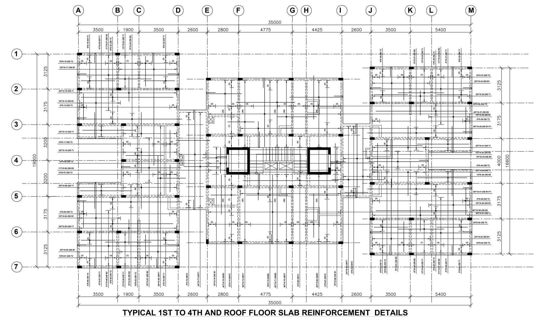
The Slab is 150mm Thick Suspended RC Slab
