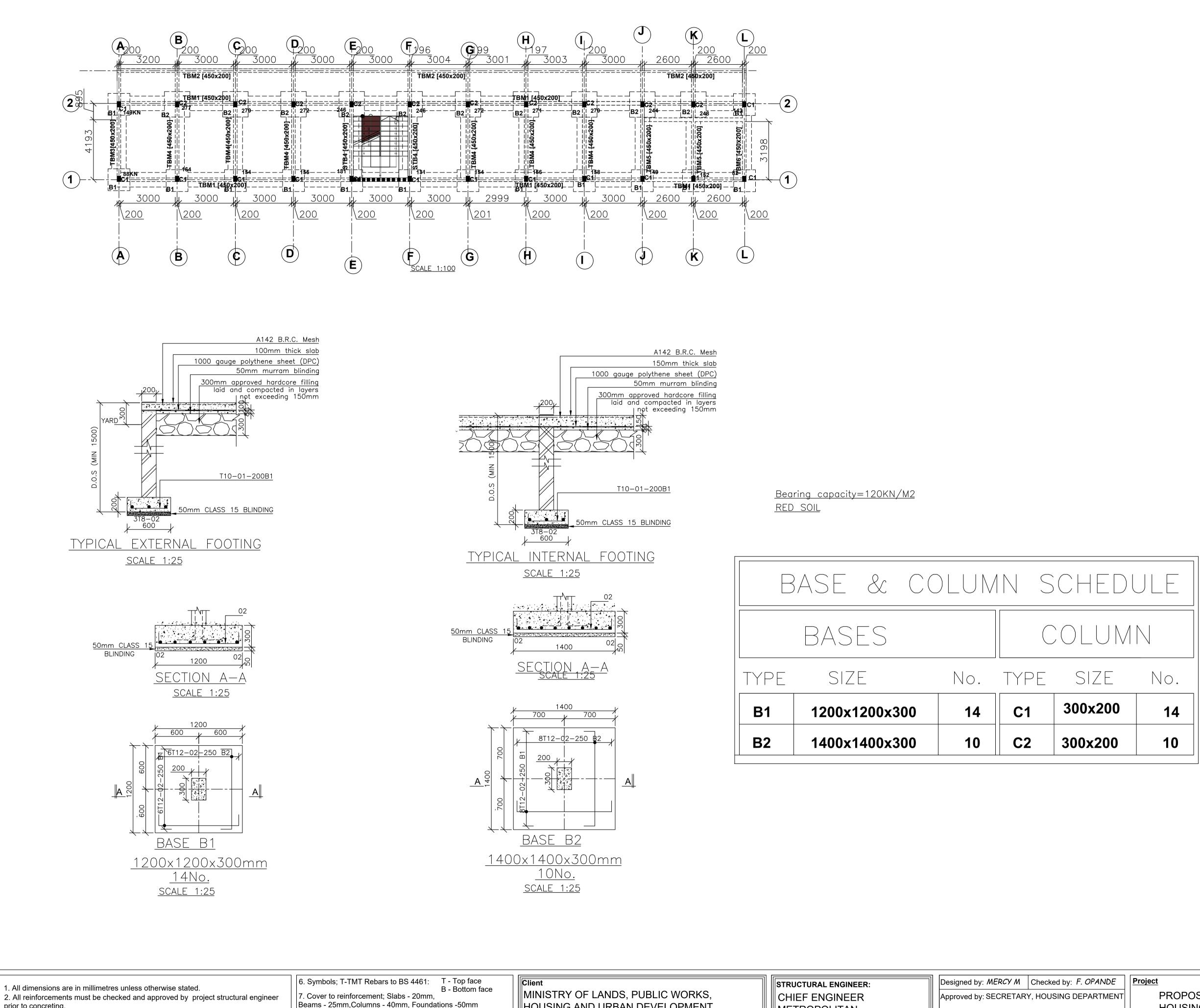
prior to concreting. 3. All reinforced concrete to be Class 25 mix and blinding concrete to be Class 15 mix. 4. Only figured dimensions to be taken from this drawing. 5. Any descripancy indimensions to be reported to the project consultants i.e architect or engineer.
