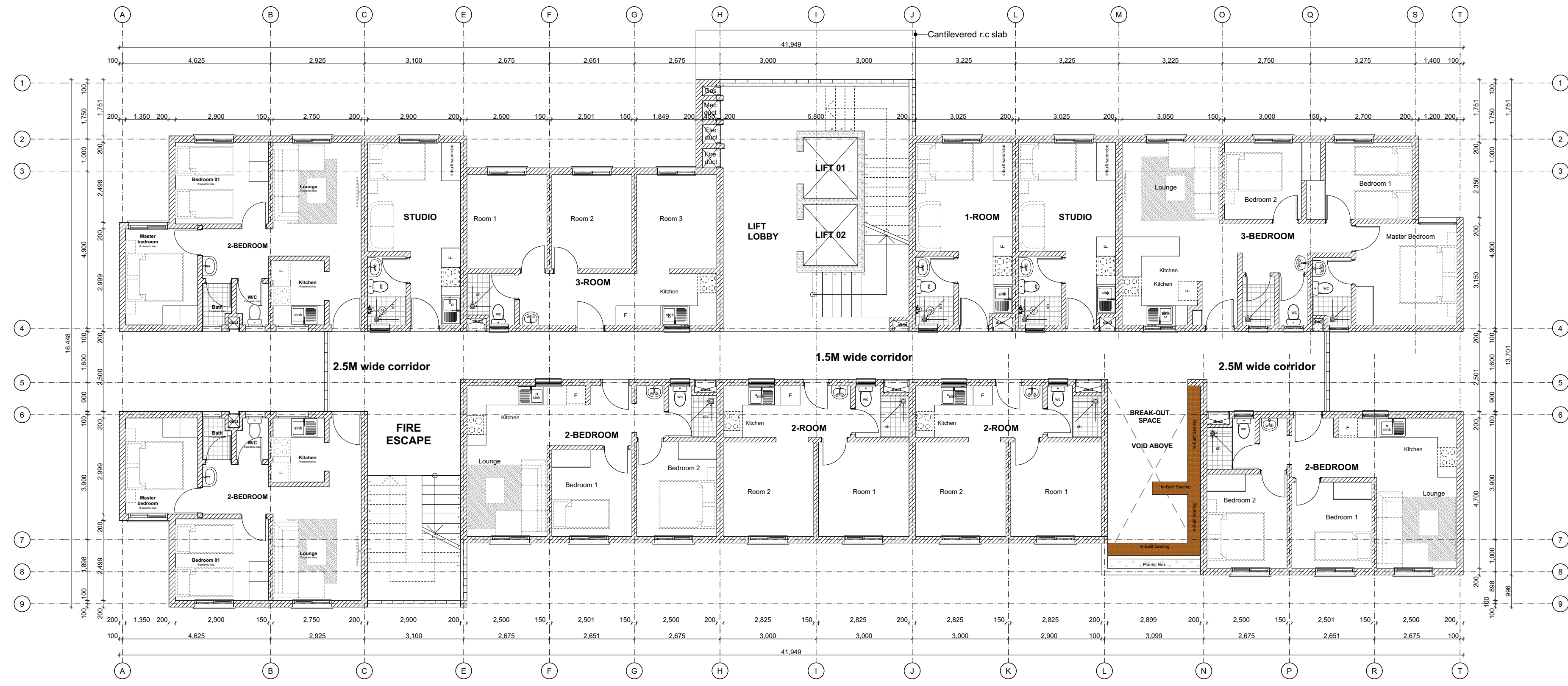
PROPOSED TYPICAL SOCIAL+ AFFORDABLE UNITS BLOCK TYPE C_TYPICAL 3RD AND 7TH FLOOR PLAN
