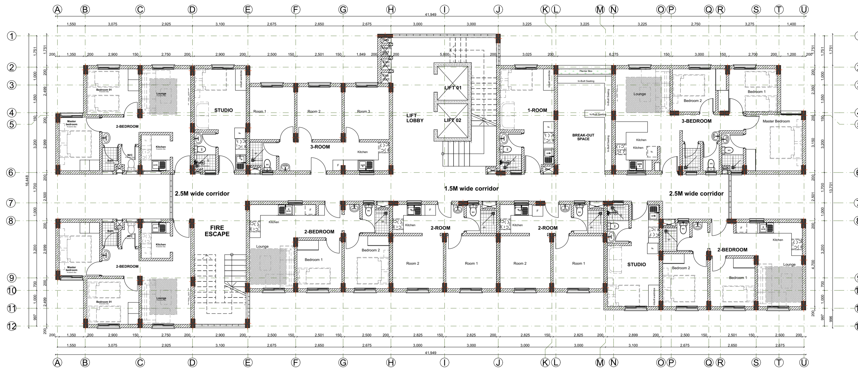
PROPOSED TYPICAL SOCIAL+ AFFORDABLE UNITS BLOCK TYPE A_TYPICAL 2ND AND 9TH FLOOR PLAN
