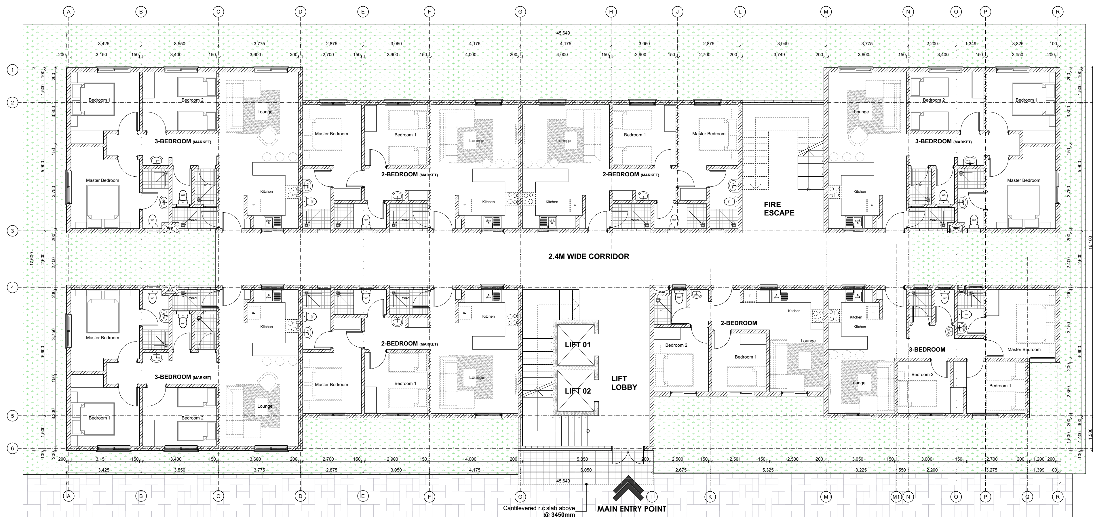
PROPOSED REVISED TYPICAL AFFORDABLE + MARKET UNITS BLOCK TYPE B_GROUND FLOOR PLAN
