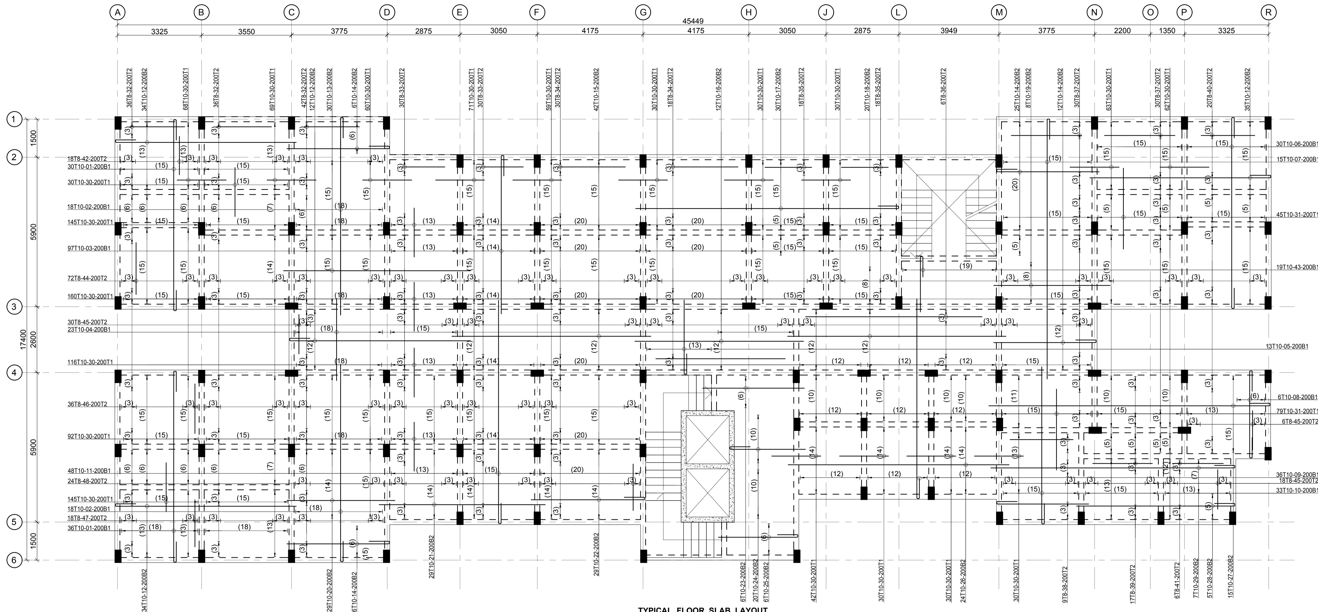
TYPICAL FLOOR SLAB LAYOUT 130 MM THICK SOLID SLAB AND 150 MM THICK SLAB IN WET AREAS SCALE 1:75
