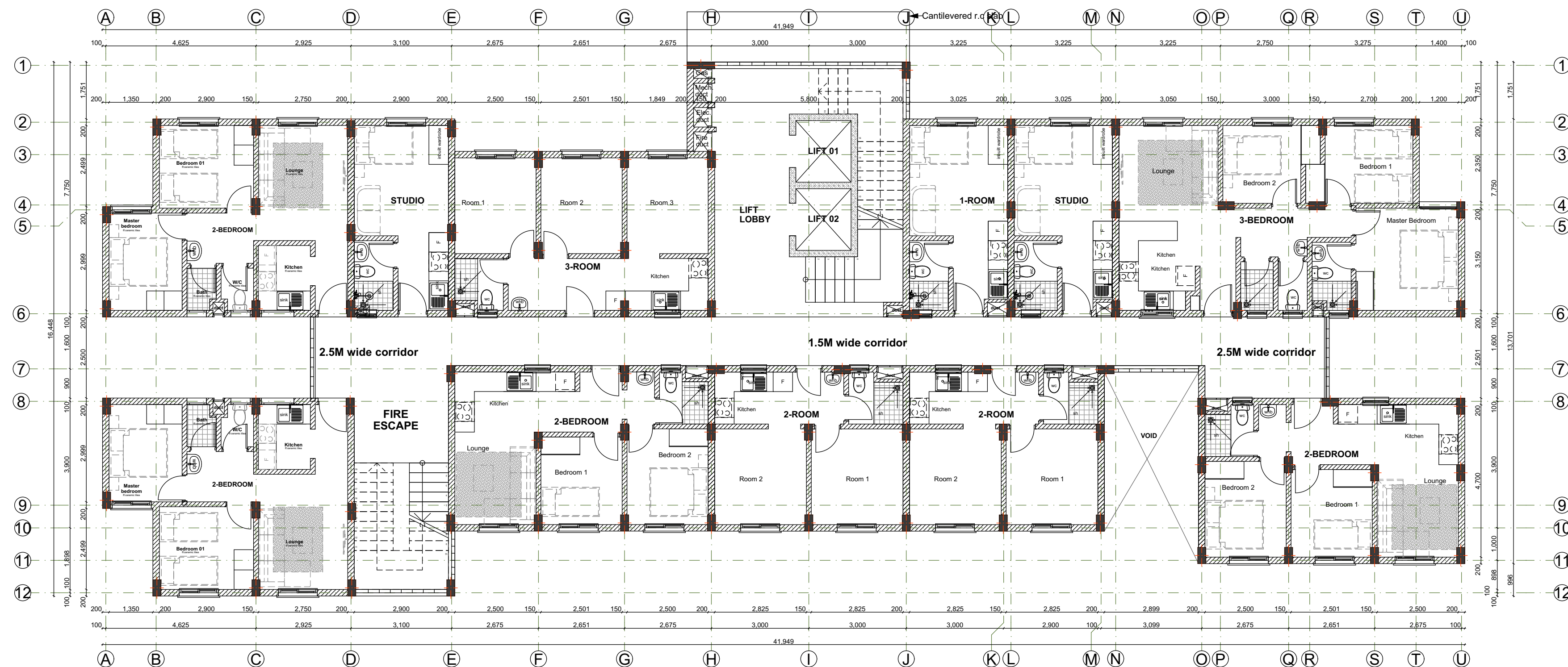
PROPOSED TYPICAL SOCIAL+ AFFORDABLE UNITS BLOCK TYPE A_TYPICAL 4TH AND 8TH FLOOR PLAN
