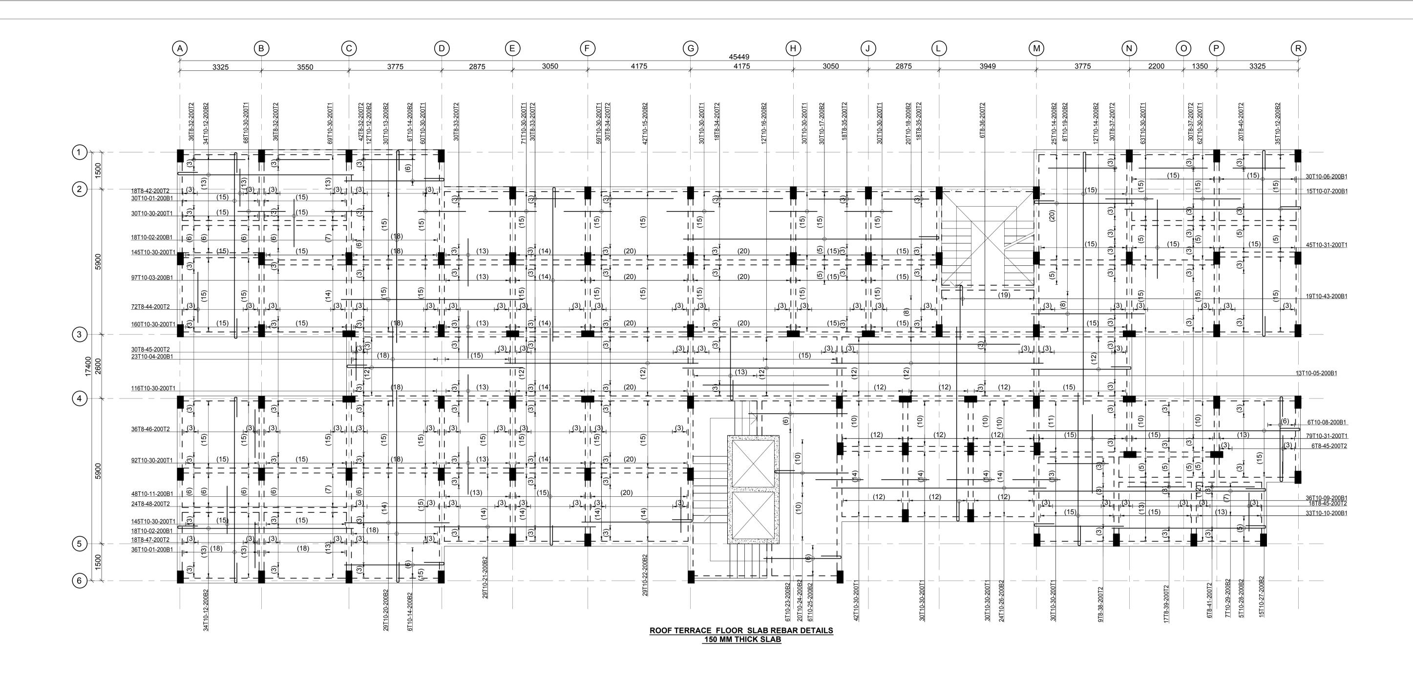
6. Symbols; T-TMT Rebars to B S 4 461 : T - Top face NOTES 1. All dimensions are in millimetres unless otherwise stated. 7. Cover to reinforcement; Slabs - 20mm, 2. All reinforcements must be checked and approved by project structural engineer Beams - 25mm,Columns - 40mm, Foundations -50mm prior to concreting. 3. All reinforced concrete to be Class 25 mix and blinding concrete to be Class 15 mix. 8. All structural steel be grade 43A.
