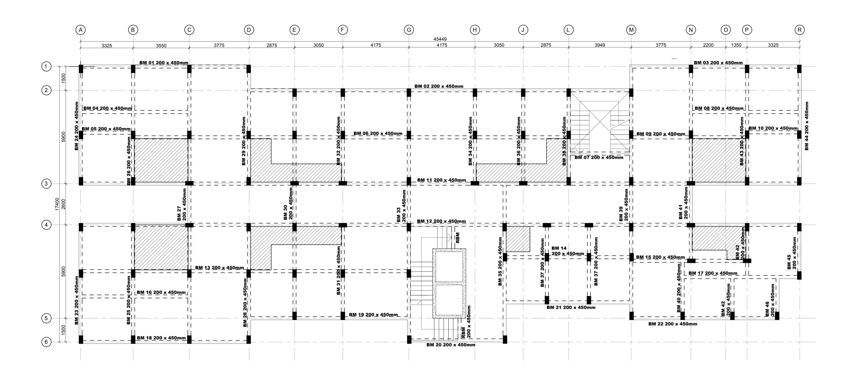
1. All dimensions are in millimetres unless otherwise stated. 2. All reinforcements must be checked and approved by project structural engineer prior to concreting. 3. All reinforced concrete to be Class 25 mix and blinding concrete to be Class 15 mix. 8. All structural steel be grade 43A.
