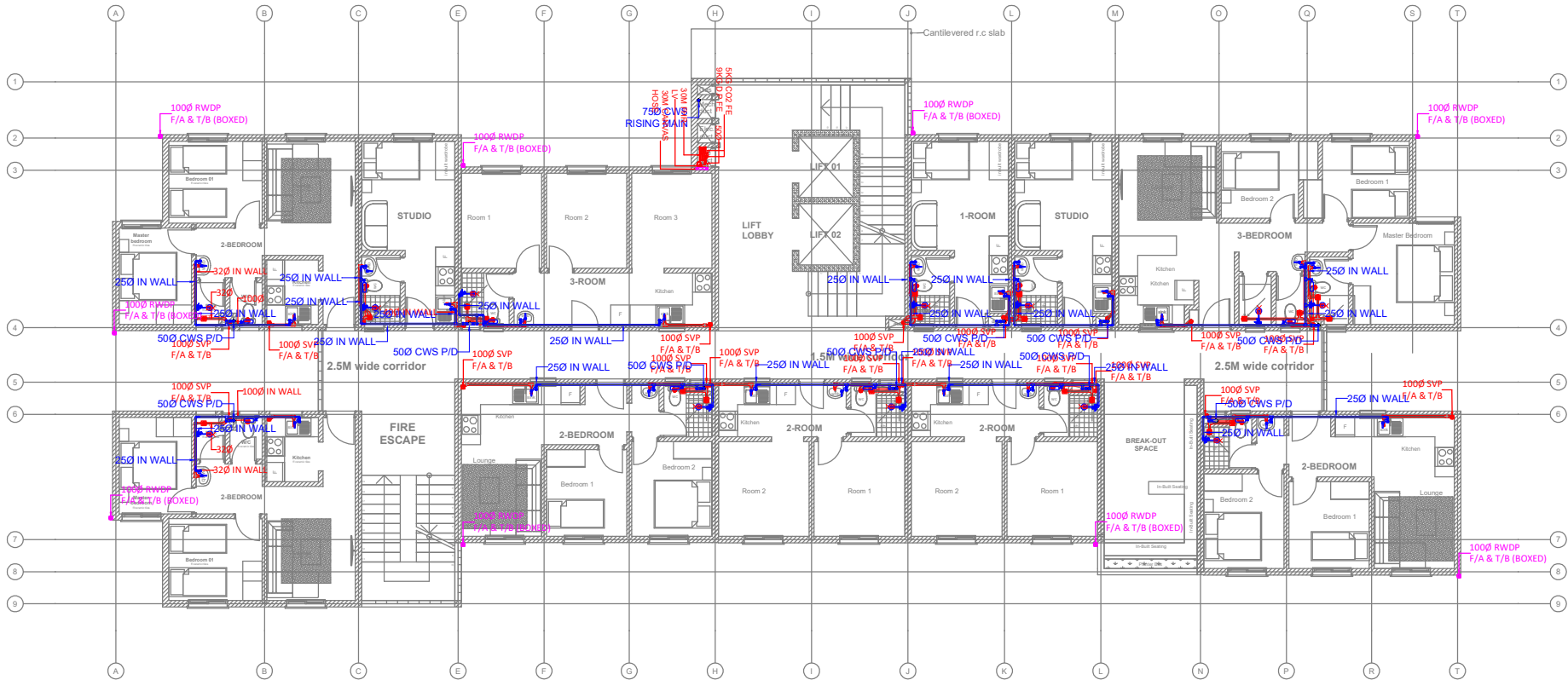
PROPOSED TYPICAL SOCIAL+ AFFORDABLE UNITS BLOCK TYPE A TYPICAL 1ST FLOOR PLAN
