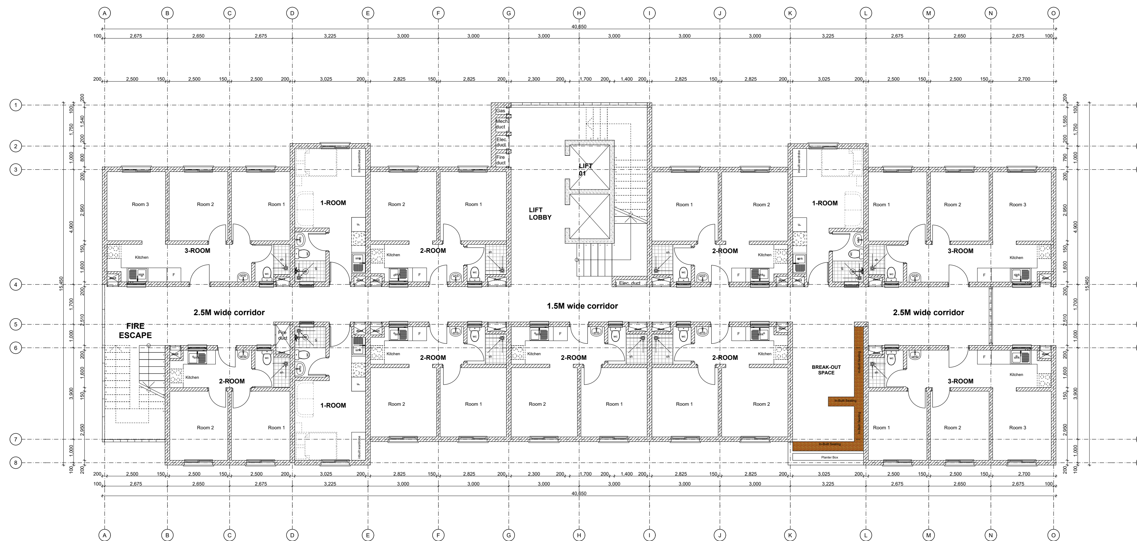
PROPOSED REVISED TYPICAL SOCIALUNITS BLOCK TYPE _TYPICAL 3RD AND 7TH FLOOR PLAN
