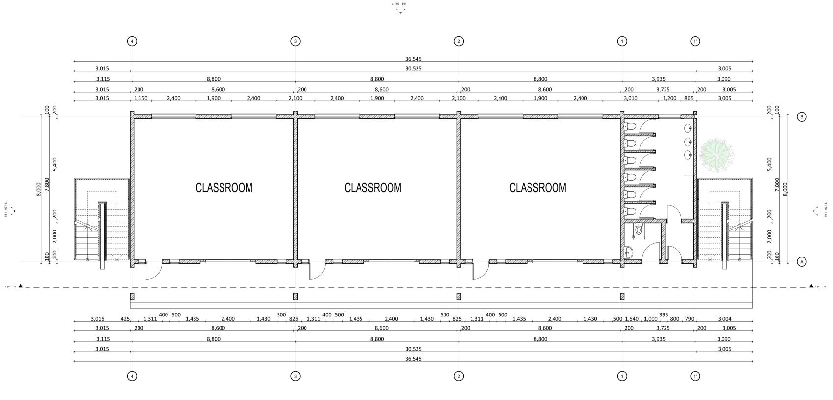
L [-2] 01 \_ Classroom Block \_ Ground Floor Plan Scale 1 : 100
