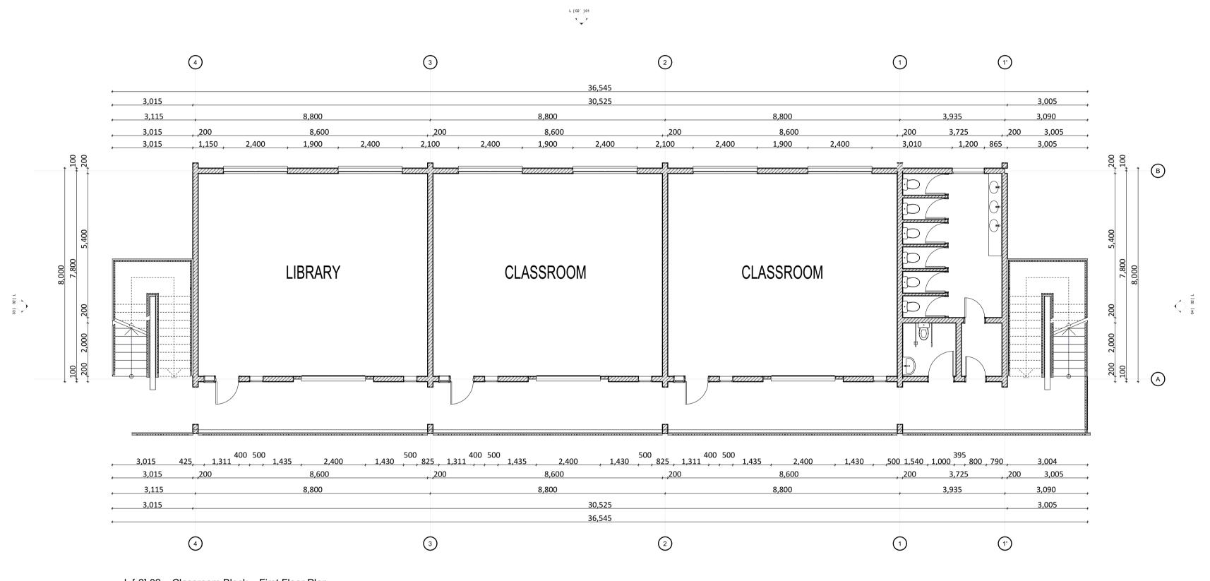
L [-2] 02 \_ Classroom Block \_ First Floor Plan Scale 1 : 100
