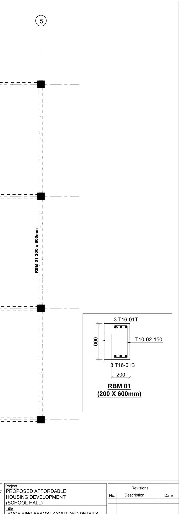
ROOF RING BEAMS LAYOUT AND DETAILS
